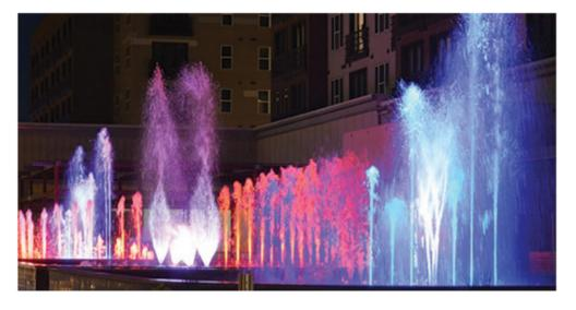
The surface area of the show fountain is approximately 3,500 square feet with nearly 52,000 gallons of water, 131 nozzles and 398 LED RGB lights capable of producing 2,000,000 colors each.
